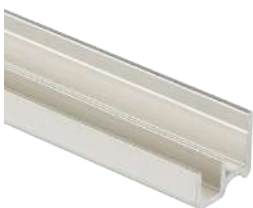
Siding Starter Clip MFG: ACL01 Material: Aluminum Size: 15 x 14.5 mm (0.59 x 0.57 in)
